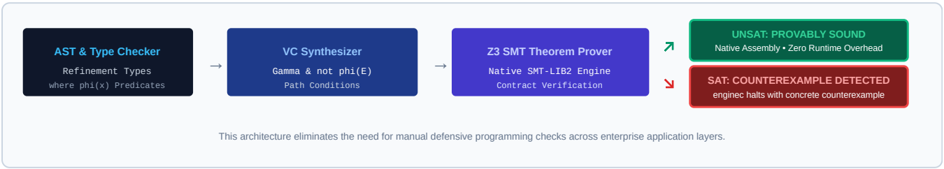
Figure 3: Compile-time formal verification pipeline embedded directly inside the enginec compiler via Z3.
